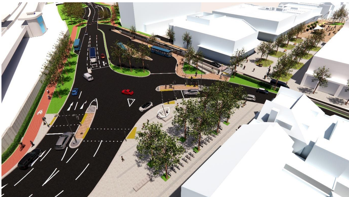
Figure 4. Conceptual plans for Saxon Street showing new highway configuration, crossings, redway links and relocated bus station. Queensway can be seen on the top right of the image.
